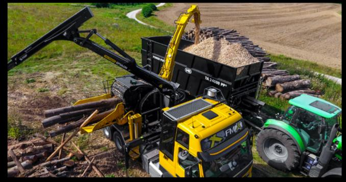
The chipper has a modified motor and charge air cooling unit, and separate cooling units for the hydraulics, gears and air-conditioning system so that the exhaust air can always be discharged reliably.
