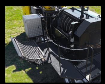
The chipper is very low maintenance thanks to the hydraulic platform, all required maintenance connections, divided screens, cutters with external screw connections and the crane for replacing the screen.
