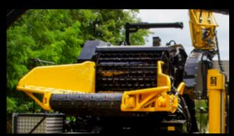
The infeed is 800 mm in height, 1200 mm wide, has two bottom feeder rollers and a large upper feeder roller with replaceable cutters. The infeed table is fitted with folding side walls to save space.
