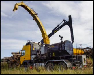
The hydraulic accelerator attached to the centre of the vehicle allows the user to load from the back and the front. The long, foldable spout allows chips to be blown precisely even under low profile doors and openings.
