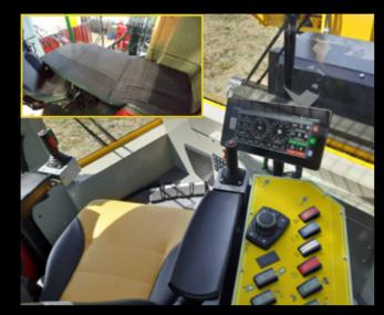
The Volvo cab offers a spacious workspace with a high degree of visibility. To control the machine, there is a large touch-screen tablet with autodidactic menu navigation available. The chipper can be moved from the operators' chair. The cabin can be fitted with sleeping accommodation as an additional option.
