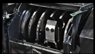
The SMC-812 has a rotor with a 200 mm cutter system, fitted with a depth limiter for variable cutting lengths of 15 - 45 mm and a large two-part screen, for the maximum throughput of the best quality.
